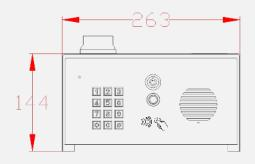
Industrial version with keypad for pedestal mount, vehicle entrances, trucks and loud industrial applications. BS316 marine grade stainless steel construction with gloss black face trim. With built in proximity reader.
