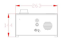
Industrial version for pedestal mount, vehicle entrances, trucks and loud industrial applications. BS316 marine grade stainless steel construction with gloss black face trim. With built in proximity reader.
